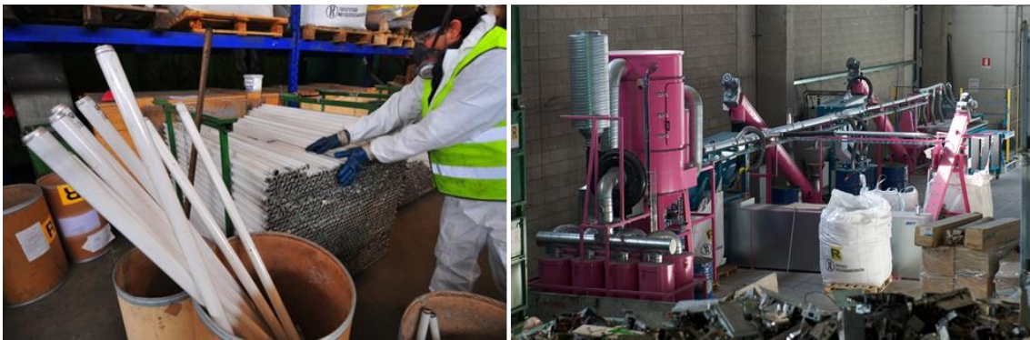
Manual sorting of the input material (left) and fluorescent lamp processing plant (right)
